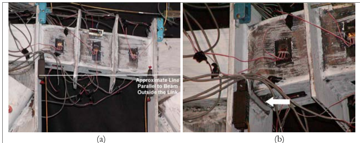
Figure 5. (a) Link deformed at 0.123 rads of rotation during cycle 19 (b) Fractured bottom flange at north end of link.
